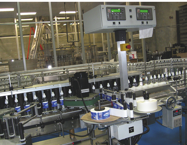
This custom-built labeler incorporates two labeling heads that can operate alternately to facilitate running short runs of bottles with different labels with minimum downtime.
