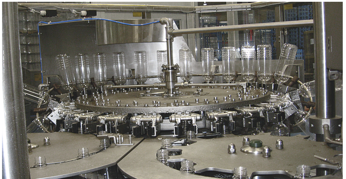
Wrapped bottles, top photo, enter the shrink tunnel. PET bottles are washed in the first module of the monobloc rinser/filler/capper, above. Next, ultra-pure water is filled by a gravity filler, after which the bottles are capped.
