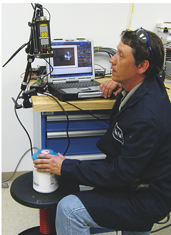
Dan Brady, Nice-Pak's electrical engineering manager, demonstrates an inspection system in his office. The camera is looking at the top of a wipes container, and the image is displayed on the computer screen on his desk.
