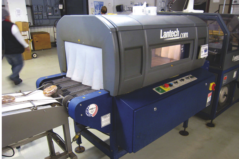
The soft-convection shrink tunnel, above, transfers heat so that it operates around 280 deg F for most polyolefins, about 70-deg less than many other tunnels.
