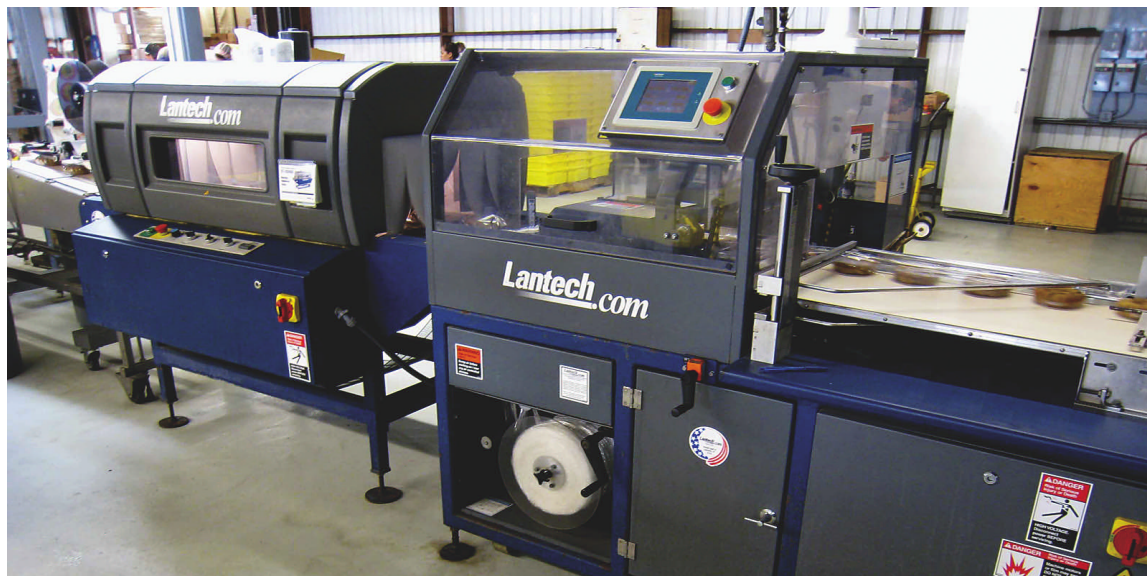
San Joaquin's new shrink-wrapping system, above, is a side-seal machine that operates at low temperatures and doesn't trim film with heat, which eliminates melted film, a problem the company experienced previously.
